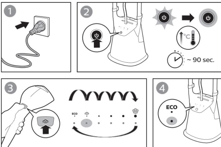
**EN** The power button flashes indicating that the appliance is heating up. When the appliance is ready for use after 90 seconds, the light turns steady.
